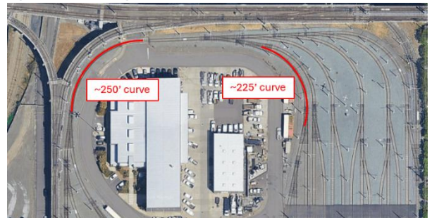
Figure 39. Turning radii at Sound Transit OMF Central
